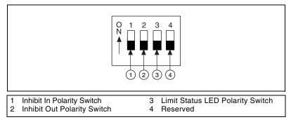
Figure 2. 4-Position DIP Switch Bank Layout
